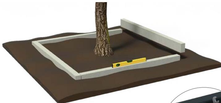
2. Place the two-piece frame on the concrete tires. Bolt the frames with the supplied materials.
