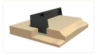
4. Then fill the inside of the retaining wall further and complete any paving.
