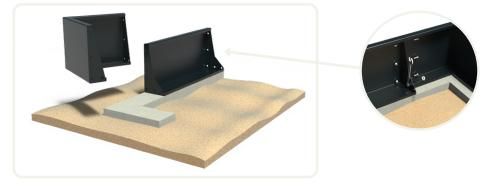
**3.** Drill holes in the load-bearing surface (the retaining walls already have holes). Then connect the retaining walls to the surface using plugs or possibly a chemical anchor. **Note!** First, tighten all bolts loosely, then tighten them one by one.
