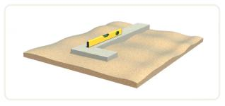
Place the retaining walls on the load-bearing surface. Bolt the elements together with the supplied materials.
