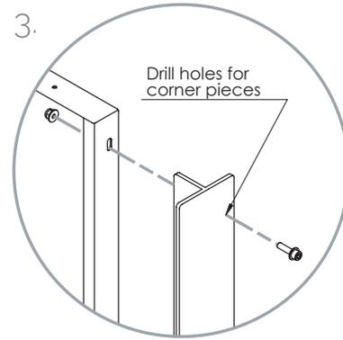
3. Thanks to the multifunctional T-shaped posts, all kinds of shapes can be created with the panels. The panels can be installed on ground level thanks to the long anchoring pins at the bottom of the T-shaped posts.
